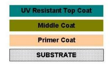
Protecto-Ezecoat 100/Protecto-Wallgard 10 is then applied over the entire surface area and allowed to dry for 4-5 hours. Equal weights of Protecto-Ezecoat 200 and 300 are mixed thoroughly and the mixture is applied by brush over the base coat.
