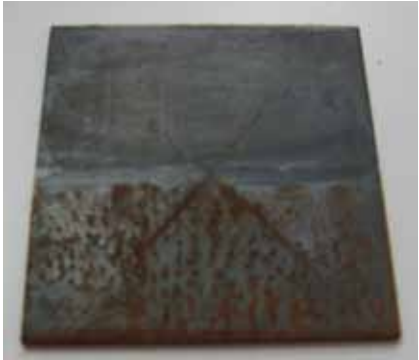
Passes 250 hours of Salt Spray Test
